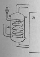
The decision will be readily understood from the subjoined cut, showing one form of the applicant's apparatus, in which E represents the boiler of the steam-engine, G a chamber in communication therewith, and P the coiled indicator pipe within the chamber. The devices for controlling the feed by means of the expansion and contraction of the liquid contained in this pipe are not necessary to an understanding of the decision, and are not shown.
