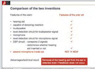
Note that the new problem (detection of the removal of the hearing aid from the ear without relying on the unpleasant occurrence of feedback) is different from the initial problem we wanted to solve ("use less battery").
